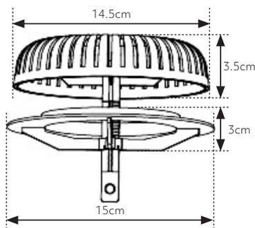
**Usage:** Can be fitted into all kinds of roofing underlay materials, including bitumen, from 0.2 – 25mm
